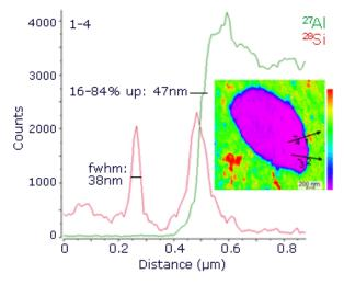
First tests on the IPREM's NanoSIMS 50L have confirmed that beam size and densities achieved with the new O- primary ion source for electropositive trace elements (alkalis, metals, REEs, uranides), are equivalent to those achieved with the Cs+ ion source for negatives secondaries. Additionally, the new source does not sputter internally, thus lifetime is now counted in months between cleaning. Finally long term current stability is excellent: below 1%
