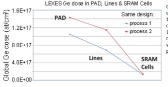
The Shallow Probe detects that both processes do not behave the same way depending on the area, and a growth loading effect is observed from pad to lines.
