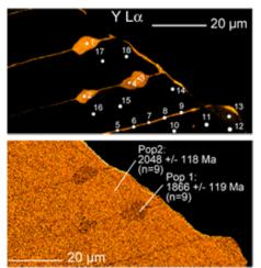
CAMECA EPMA instruments have been widely used for chemical dating of monazite.
