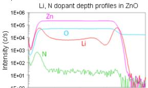
Li and N in-depth distribution could be successfully characterized, as shown here, demonstrating that the IMS 7f-Auto delivers profiles with excellent detection sensitivity and high depth resolution, which is essential for LED technology.
